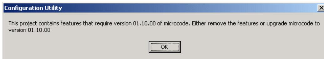
Following this warning message, the system generates an error report. (In this example, the project attempted to assign Latching Supervisory to P:01 C:01 D:002 and Latching Tamper to P:01 C:01 D:003. These types are not supported in CPU version 01.00.00. Also, the project included a panel type that is invalid.
